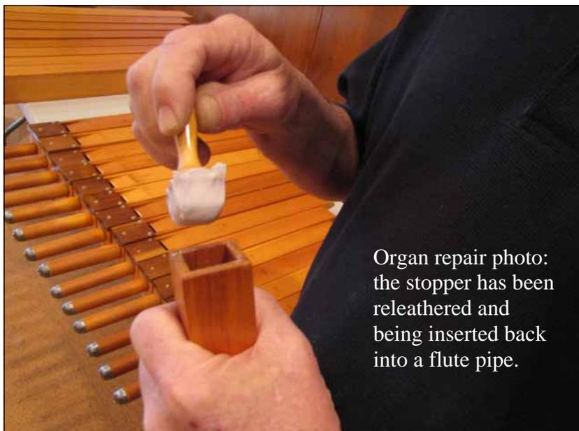
Organ repair photo: the stopper has been releathered and being inserted back into a flute pipe.
